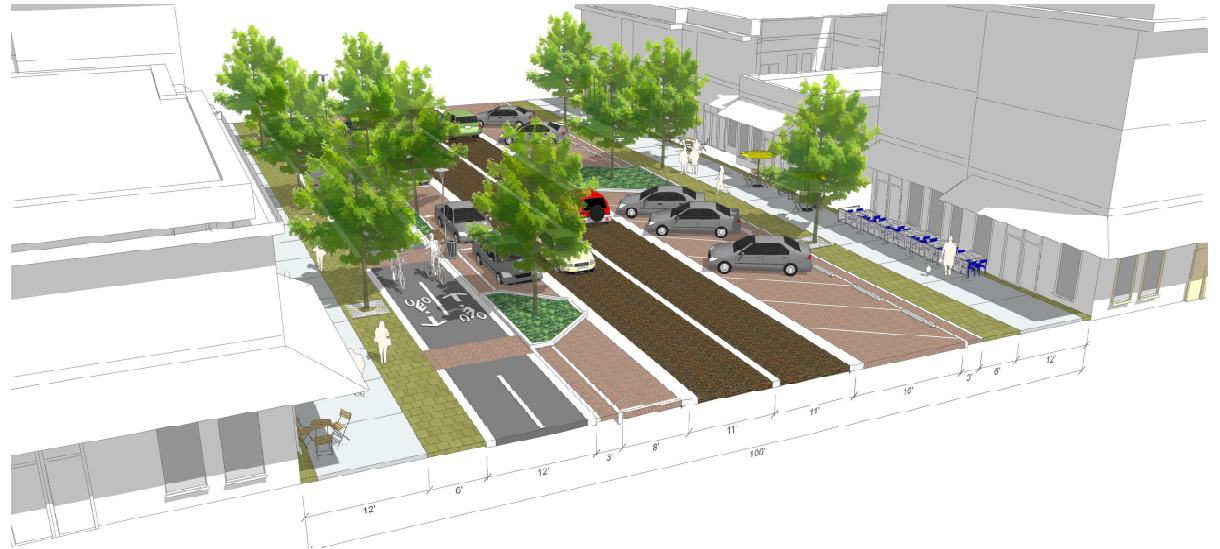
Main Street additional design concept with a two-way bikeway on the north side of the street.
