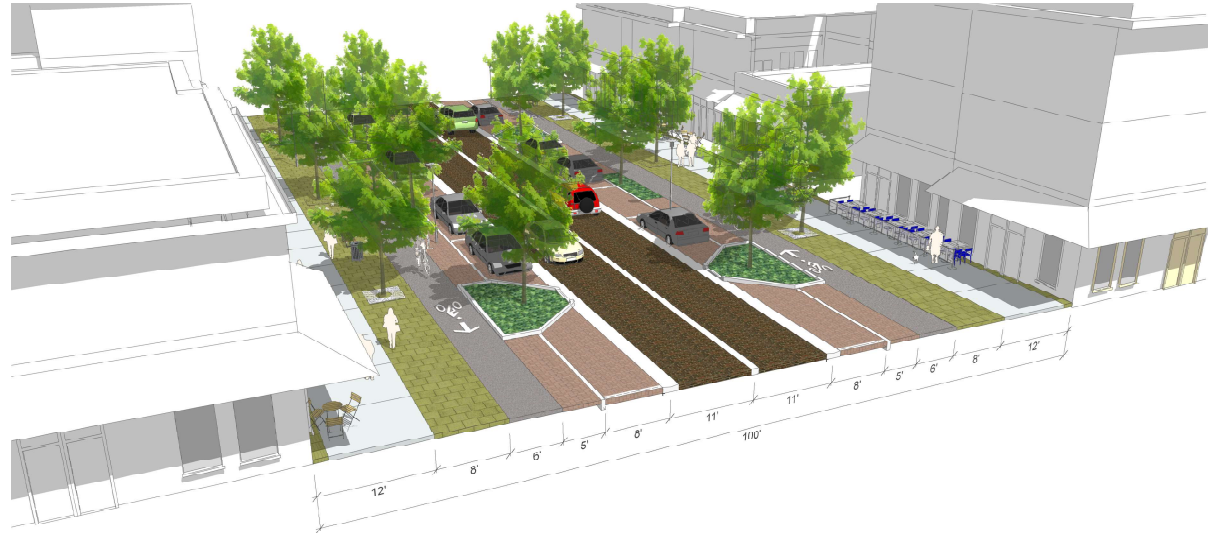
Main Street initial design concept with one-way bikeways on each side of the street.
