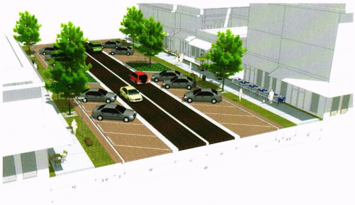
In some locations the Main Street right of way is 95 so the furnishing zones are narrowed. Sidewalk, parking, and vehicle travel lane dimensions are not changed.
